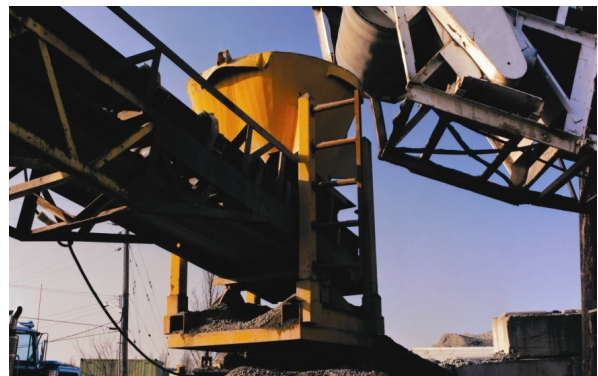
↑ Quarry conveyor tail drum assembly
