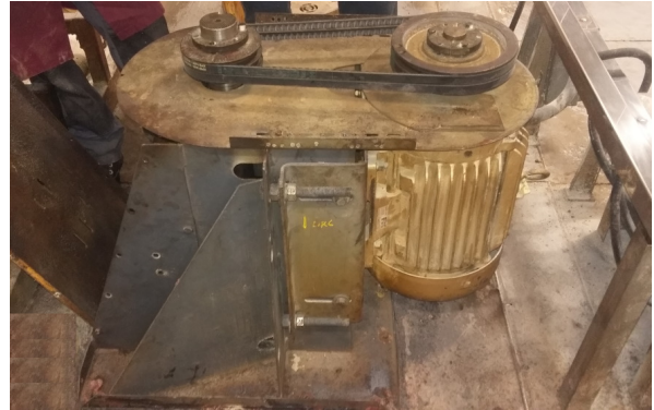
↑ Oven Re-Circulation Fan Unit
